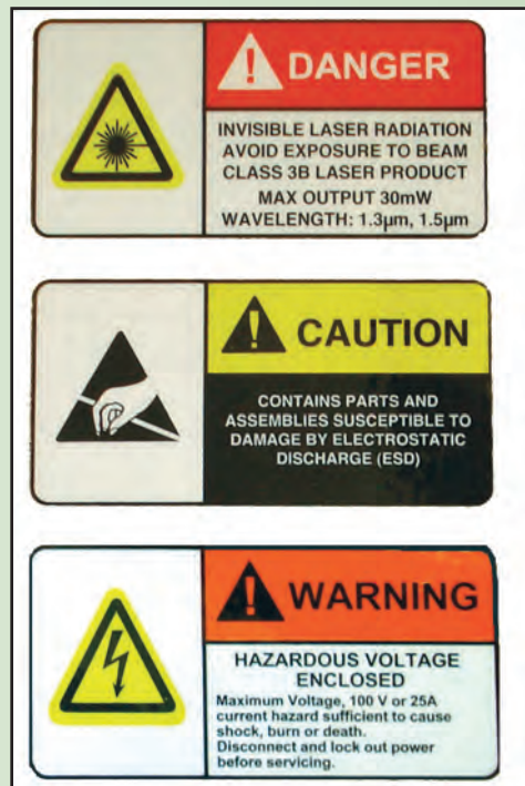
Labels after being subjected to extreme testing.
